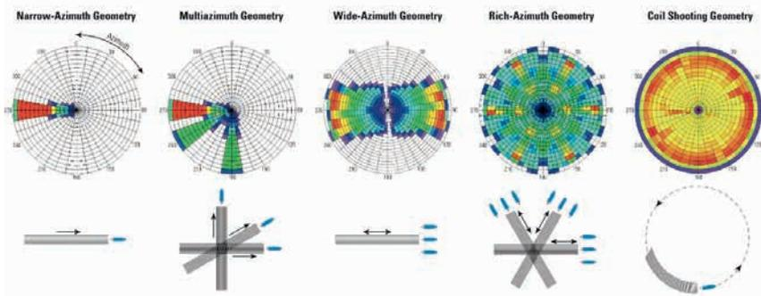
**Figure 2** Rose diagrams obtained from different variants of streamer acquisition.
