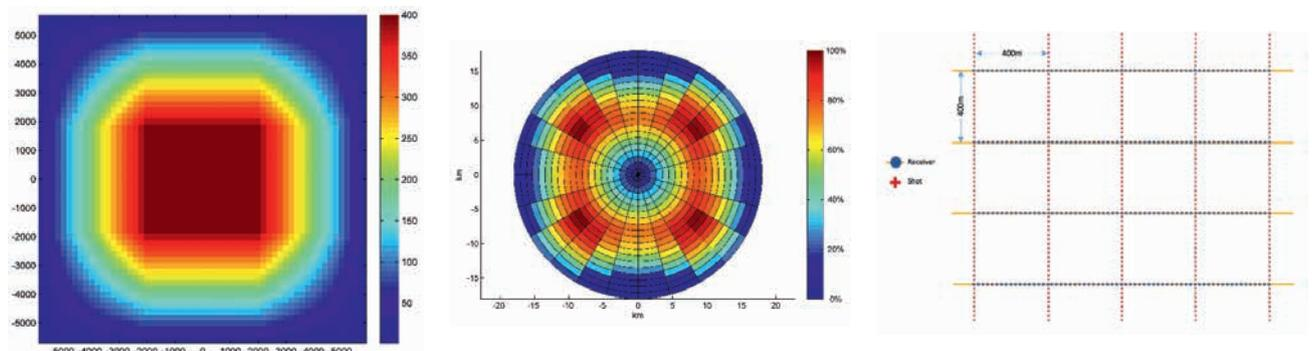
**Figure 4** From top to bottom – seismic coverage, rose diagram and acquisition geometry zoom with Midwater Stationary Cable (20 8-km long cable spaced by 400 m; orthogonal shooting with 25-m shot point interval and 400 m).
