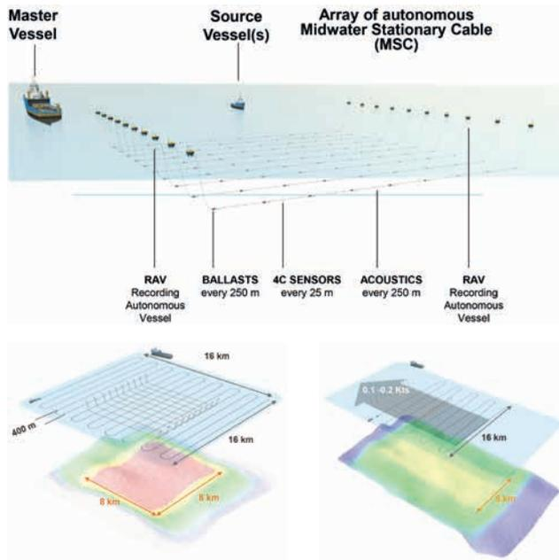
**Figure 3** From top to bottom to bottom – Midwater Stationary Cable array and operating methods: patch shooting (left) and progressive shooting (right).
