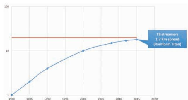
Figure 1 Maximum number of towed streamers behind a seismic vessel vs. time.
